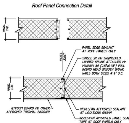
Insulspan SIP roof joint sealing details include two levels of redundancy to prevent air movement within the joint: 1) joint sealant applied to the vertical face as well as the top and bottom face of the 2x wood spline used to join the SIPs and 2) panel seal tape applied to the underside of SIP roof joints. As well, a sealant is applied to the top edge of OSB skins to seal the top surface of the SIP joint.
